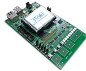
Figure 1. JTAG Functional Test (JFT) based sensory board.
