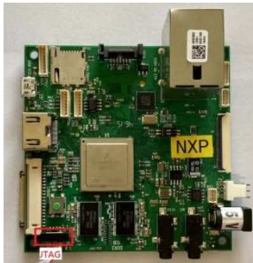
Figure 10. System under study based on an NXP designed automotive board.
